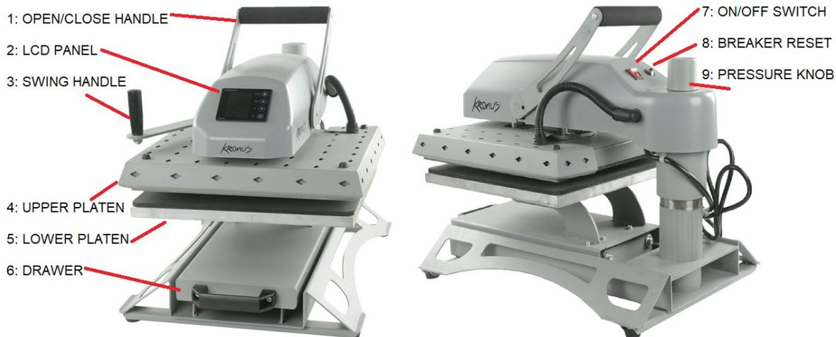
1. Open/Close Handle. Pull down to start heat pressing. Pull up to open.
